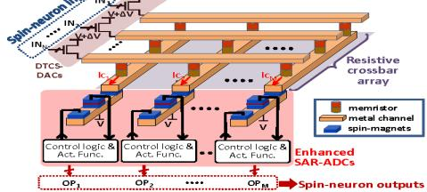
Figure 2: Array of spin-neurons
