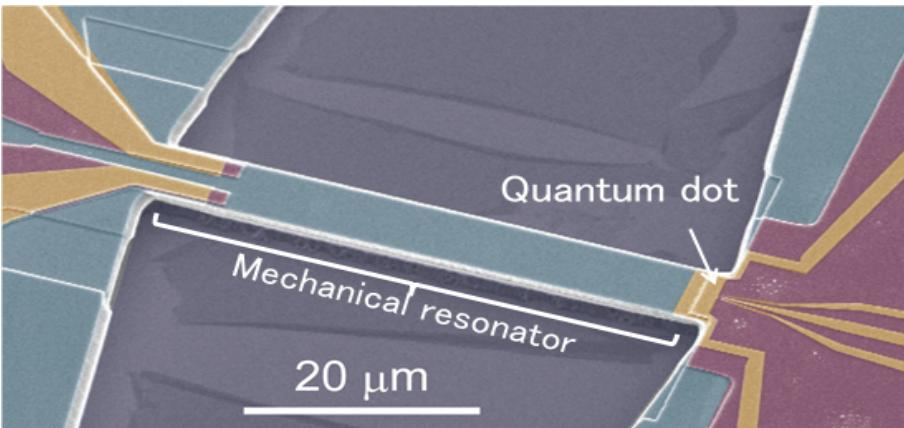
Fig: Fabricated mechanical resonator and quantum dot hybrid device. The resonator motion can be detected through the change in the conductance of quantum dot.
