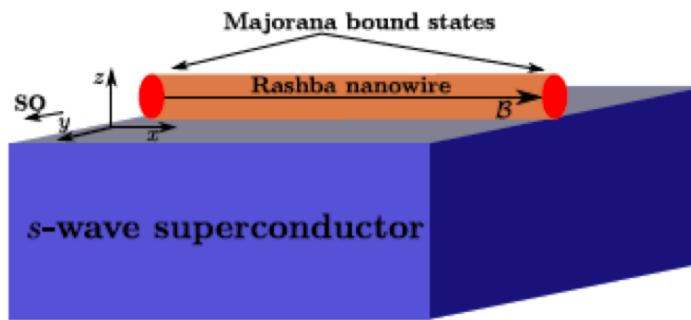
$$H_0 = \frac{p_x^2}{2m} - \mu - \frac{\alpha_R}{\hbar} \sigma_y p_x + \frac{g\mu_B}{2} \sigma_x B$$
